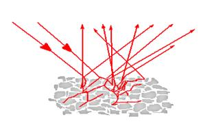
Highly reflective particles (e.g. magnesium oxide, plaster paper fibers)
