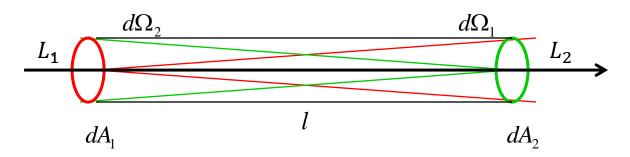
Flux leaving surface 1 must be equal to flux arriving on surface 2  $L_1 d\Omega_1 dA_1 = L_2 d\Omega_2 dA_2$
