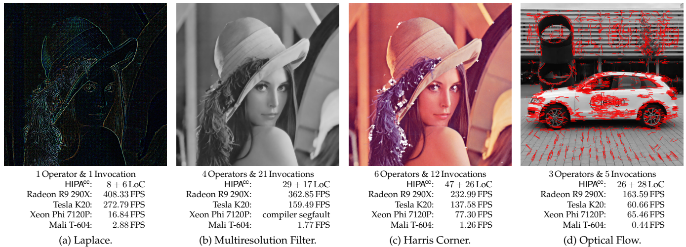
Figure 10: Algorithms in HIPA cc : edge detection (a), multiresolution processing (b), corner detection (c), as well as optical flow (d). Listed are the number of operators required for the algorithms as well as the total number of operator invocations. The (X + Y) LoC denote the DSL parametrization (X) and the algorithm implementation (Y) in DSL code. All benchmarks were performed using OpenCL on 4K UltraHD (3840 × 2160) images.
